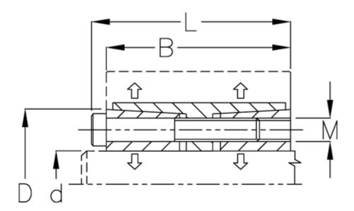
B mm = 155d H8 mm = 360D mm = 455Fit tolerance = Aksel h8, Nav H8 F kN torque = 2783.0L mm = 177M mm = M22P N/mm2 surface pressure on shaft/hub = 142 Surface roughness = R? ?  $3.2 \mu n$ T N m torque = 501000Ts N m bolt tightening torque = 930.0
